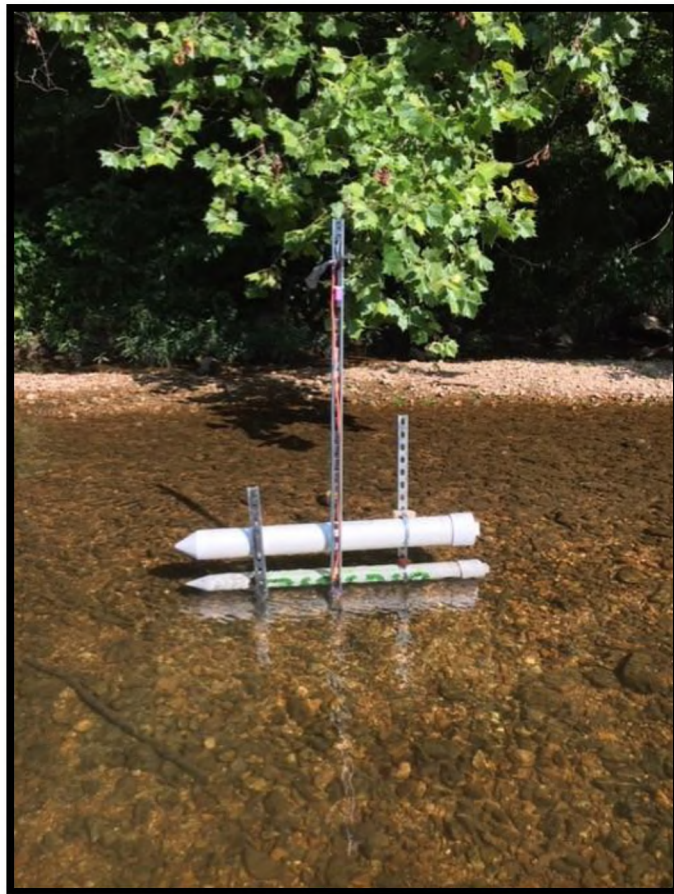
Figure 3.9 Samplers Oriented Upstream
