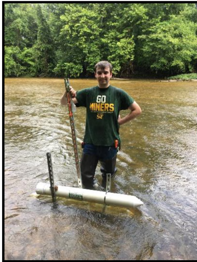
Figure 3.7 Sampler Stability Testing
